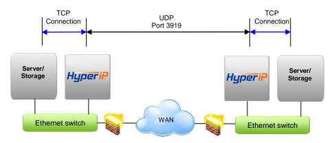
HyperIP terminates TCP connections locally and tunnels the data between HyperIPs using UDP port 3919. Network devices filtering IP traffic in the data path between the HyperIPs must be configured to allow UDP port 3919.
