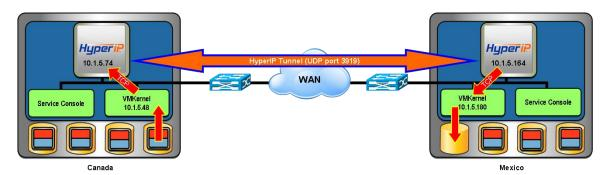
The HyperIPs must be configured to intercept VMotion traffic for these sites (see Appendix A for HyperIP configuration) and the VMkernel routing tables need to be modified to direct the traffic to the HyperIPs. Local route statements are added to the VMkernel using the local HyperIP as the gateway to the remote VMkernel. You must be logged into the ESX server with the authority to make VMkernel routing changes.
