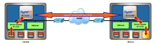
The HyperIPs must be configured to intercept VMotion traffic for these sites (see Appendix A for HyperIP configuration) and the ESX routing tables need to be modified to direct the traffic to the HyperIPs. Local route statements are added to each Service Console using the local HyperIP as the gateway to the other Service Console. You must be logged into the ESX server with the authority to make routing changes.
