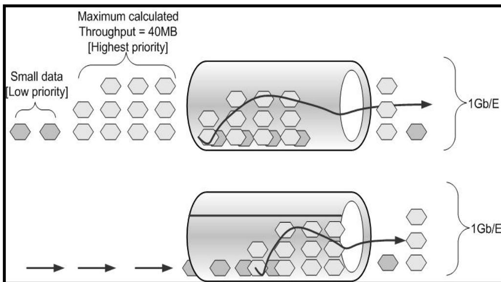
**Figure 4. Representation of traffic shaping by priority class**
