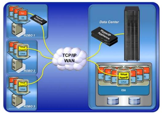
The end result is that Virtual HyperIP provides 80-90% utilization of the available bandwidth between data centers and/or ROBOs up to OC12 rates versus the 5 to 30% utilization that is common. Applications will see up to 10 times the performance and can see an effective bandwidth throughput that can be actually *greater* than the rated throughput (depends on the effective compression ratios).
