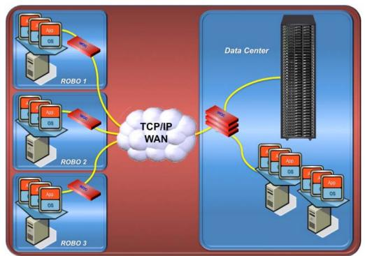
servers containing proprietary WAN acceleration software. The WOCs are deployed in the data center and at each ROBO while working together to intercept and accelerate traffic flows between ROBO users and the data center servers. Most WOCs are designed to perform some or all of the following operations:
