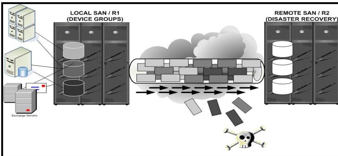
**Figure 2. SRDF/A topology with latency, packet drops, and oversubscription**
