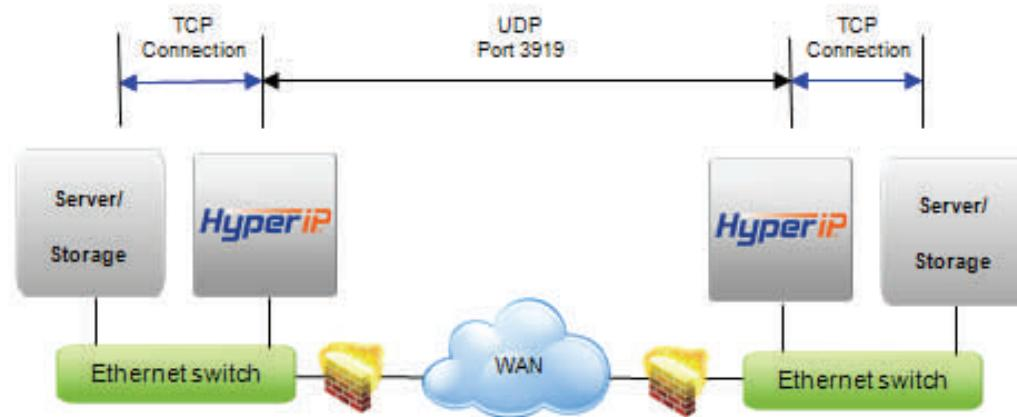
HyperIP terminates TCP connections locally and tunnels the data between HyperIPs using UDP port 3919. **Network devices filtering IP traffic in the data path between the HyperIPs must be configured to allow UDP port 3919.**
