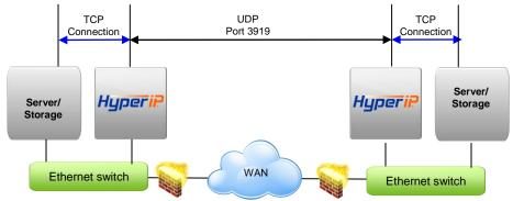
HyperIP terminates TCP connections locally and tunnels the data between HyperIPs using UDP port 3919. Network devices filtering IP traffic in the data path between the HyperIPs must be configured to allow UDP port 3919.
