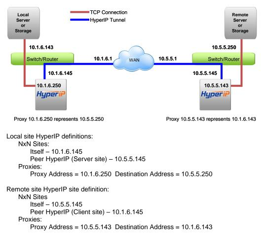
The storage clients or servers use the proxy address where the remote client or server would be set in their configuration. For example, the local server transfers a file to the remote server using ftp with a command similar to the one below:
