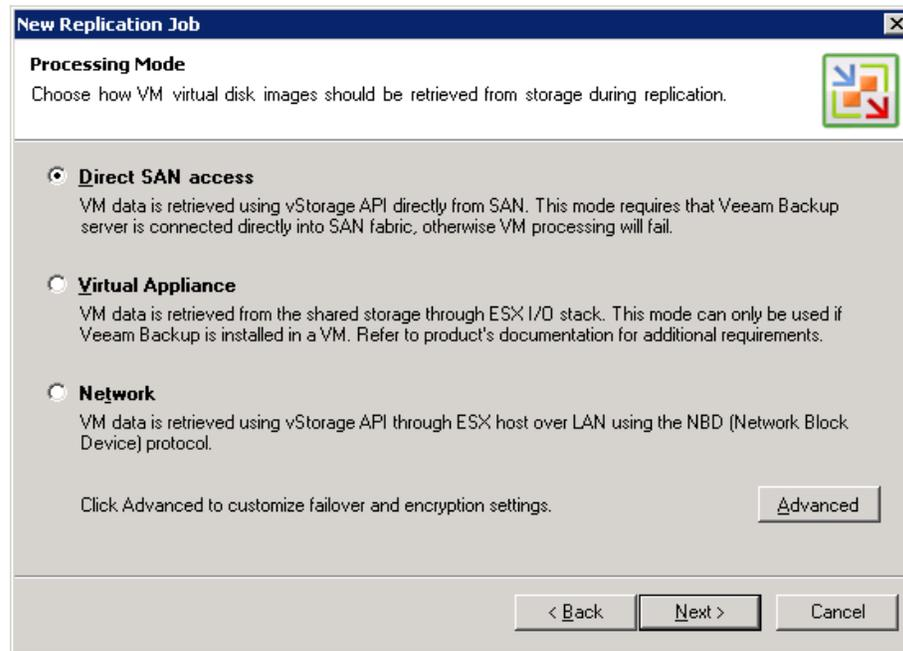
The processing modes determine how data will flow between the source ESX(i) host and the Veeam Backup Server. HyperIP resides between the Veeam Backup Server and the remote (across the WAN) ESX(i) or Linux host.
