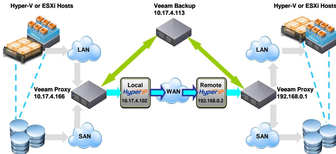
In the Veeam Proxies, add a persistent host route to the remote proxy with HyperIP as the gateway. An example for the IP addresses in the above drawing:
