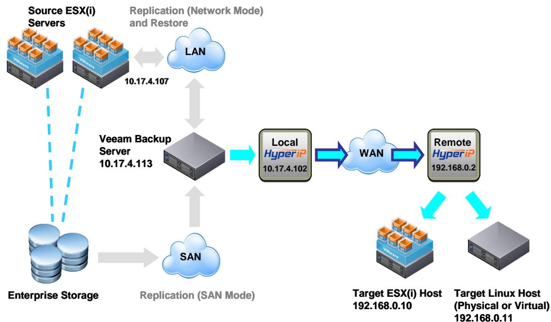
In the Veeam Backup Server, add a persistent host route to the Target ESX(i) or Linux host with HyperIP as the gateway. An example using the IP addresses in the above drawing:
