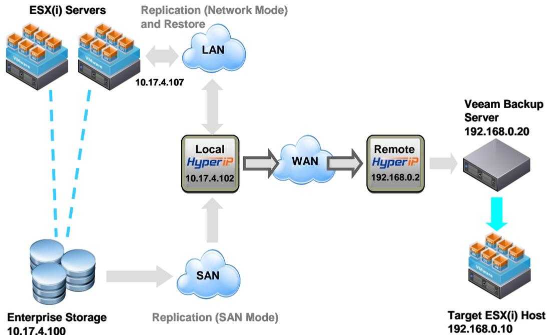
In The Veeam Backup Server, add a persistent host route to the remote ESX(i) host with HyperIP as the gateway. An example using the IP addresses in the above drawing:
